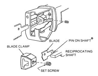
\* NOTE: A special pin holds the blade clamp on the reciprocating shaft to prevent the clamp from coming off when set screw is loosened
