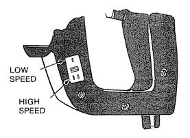
LOW SPEED (Move slide switch to show (I) bar). For cutting sheet metal, metal pipe, metal conduit, etc
