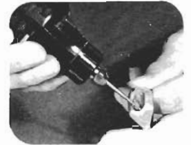
Grind cast rings
