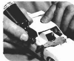
Grind off excess material
