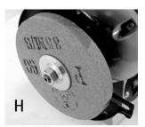
There is a left and right tool rest. When in actual use, the tool rests should be adjusted to within 1/8" (3.2mm) of the grinding wheel or other accessory being used. Follow the illustrations to remove/install the tool rest. The Grinding Wheel is accessed by removing the Eye Shield and Tool Rest and the Wheel Guard.
