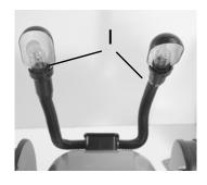
Your Bench Grinder may include adjustable lights. Lights can provide visual aid when using the Bench Grinder (Figure I)
