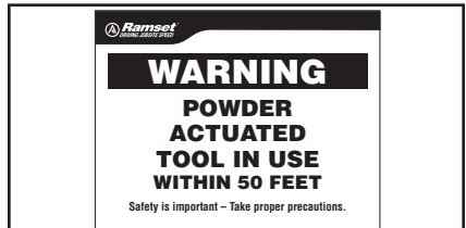
ALWAYS POST WARNING SIGNS
