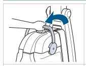
1. Remove the Dirty Water Tank. Pull handle to upright position and lift up to remove.
