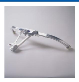
AC78 QuickClick™ Stabilizer spans 44 in and provides a standoff of 10 in. Requires no tools to attach to ladder. Spring-loaded locking latch makes it easier and quicker to install/remove than any other stabilizer on the market. Mar-resistant rubber end caps protect the work surface.
