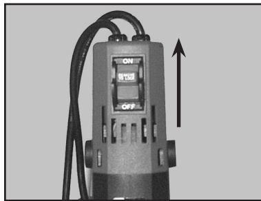
(E) Turn the motor ON
