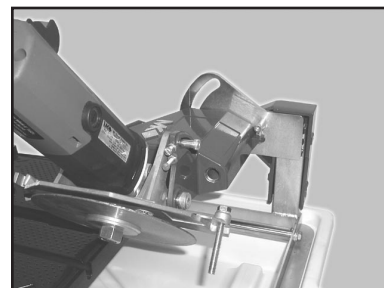
(H) Repeat steps A to G until Blade is even across all points of Square
