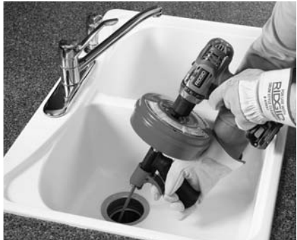
Figura 8A – Power-Spin Powered By Battery Drill
